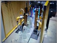
X-Pattern flame treat can be used in-line before PYROSIL, or in a modular conveyorized setting.
